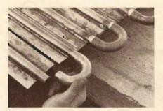
Earlier version used strips of V-5 grooved metal held together with sheet metal screws. You may find this easier to keep flat while soldering.
