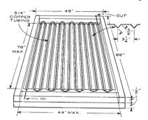
Number and spacing of V grooves can be varied (compare drawing and photo). Shown: 4-by-8-by-1½" beadboard panels, 17 tubes of 80-by-¾"
