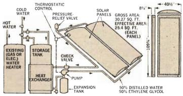
changer is outside storage tank to prevent possible contamination of water by toxic ethylene glycol. Grumman, the maker, says two collectors give 50 gal, of hot water per day. \$995.
