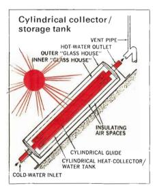
Heating of water between SAV's heat collector/water tank and guide causes siphon circulation in direction of arrows. Collector heats water directly, uses no heat exchanger or pump. Cold-water reservoir must be above top of collector in natural-circulation systems such as this. Price: \$350 per collector.
