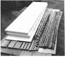
copper; 16 sets of copper return bends and couplings, and plywood (optional). Also needed: a 78-by-43-in. sheet of 24-qauge galvanized metal, and fiberglass.
