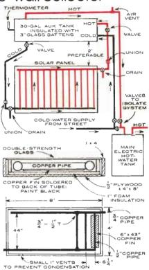
black. Finally, mount the piping in a 4'-by-8' box made of  $\frac{5}{8}$ " exterior plywood to which you have added 1-by-4 sides. Paint the box and line the bottom and sides with one inch of urethane-foam insulation. A 30-gallon galvanized water tank was ceiling mounted, wrapped in four inches of fiberglass insulation, and boxed with  $\frac{1}{4}$ " plywood.
