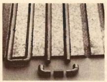
Pipes are soldered into V grooves 4 in sheet-metal plate. If the copper return bends are unavailable, use street ells and couplings, as here.
