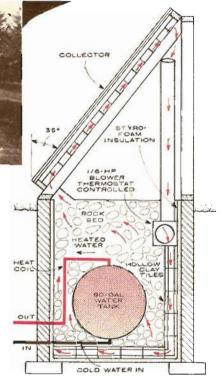
panels of common window glass, with 3/8" air separation for each section. The collector is oriented due south at  $35^{\circ}$  from vertical, the proper angle for his latitude.
